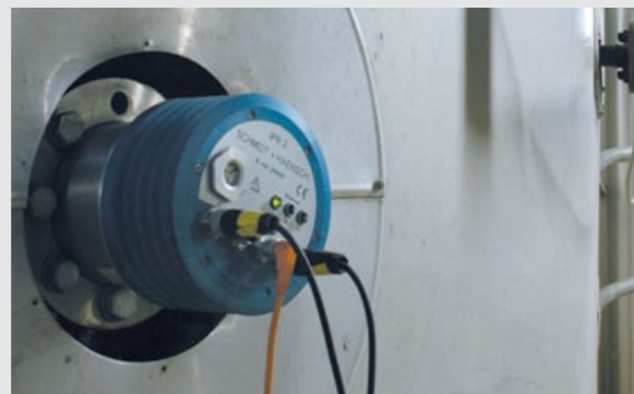
Installation in crystallizer (vessel flange) Teflon bypass for high corrosive liquids and semiconductor processes
